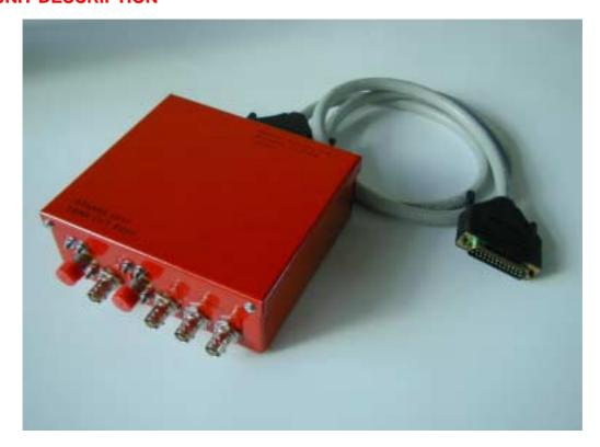
As may be seen from the above photograph, the Western Avionics 3910 FOFE Adapter unit is manufactured within a aluminium case, with all 3910 Optical, 3838 electrical, and Trigger-in and Trigger-out connections on one face, and host interface connector and LED power indicator on the opposite face.
